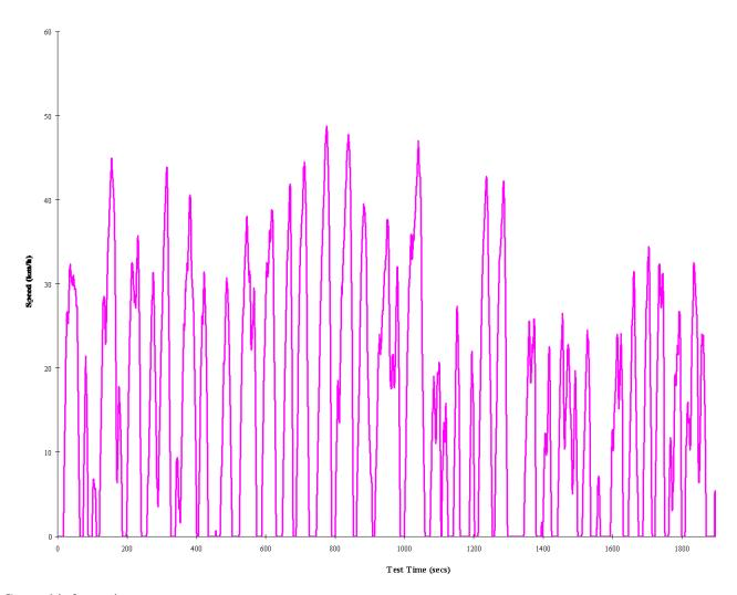
General information The overall length of the test is 2,281 seconds and the nominal distance covered is 8.92 km. Test cell ambient temperature for duration of test =  $18^{\circ}C \pm 2^{\circ}C$
