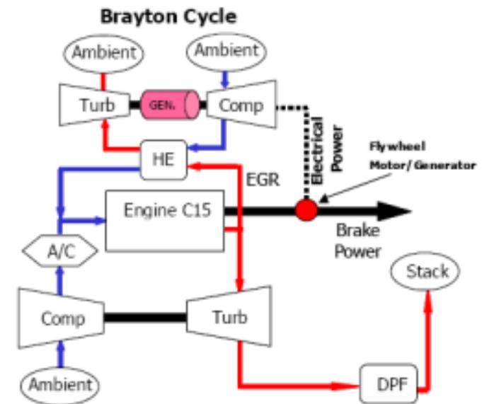
Picture: Caterpillar layout for HECC HPL EGR waste heat recovery system – Brayton<sup>1)</sup>
