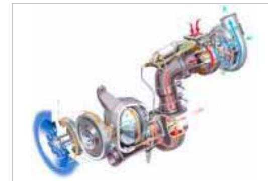
Picture: Scania turbo compound system Source: [www.scania.com](http://www.scania.com)
