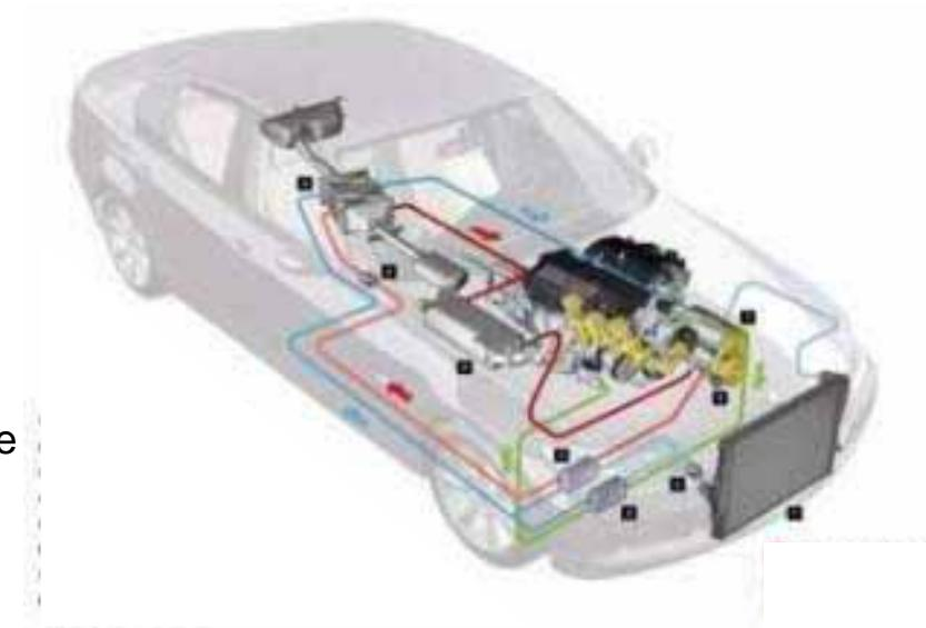
Picture: Turbosteamer in vehicle BMW 3-series; layout concept<sup>1)</sup>
