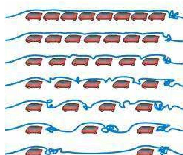
**As the main advantage of platooning is that it reduces drag, CO<sub>2</sub> benefit is highest at higher speeds where it can reach 20 – 25%**
