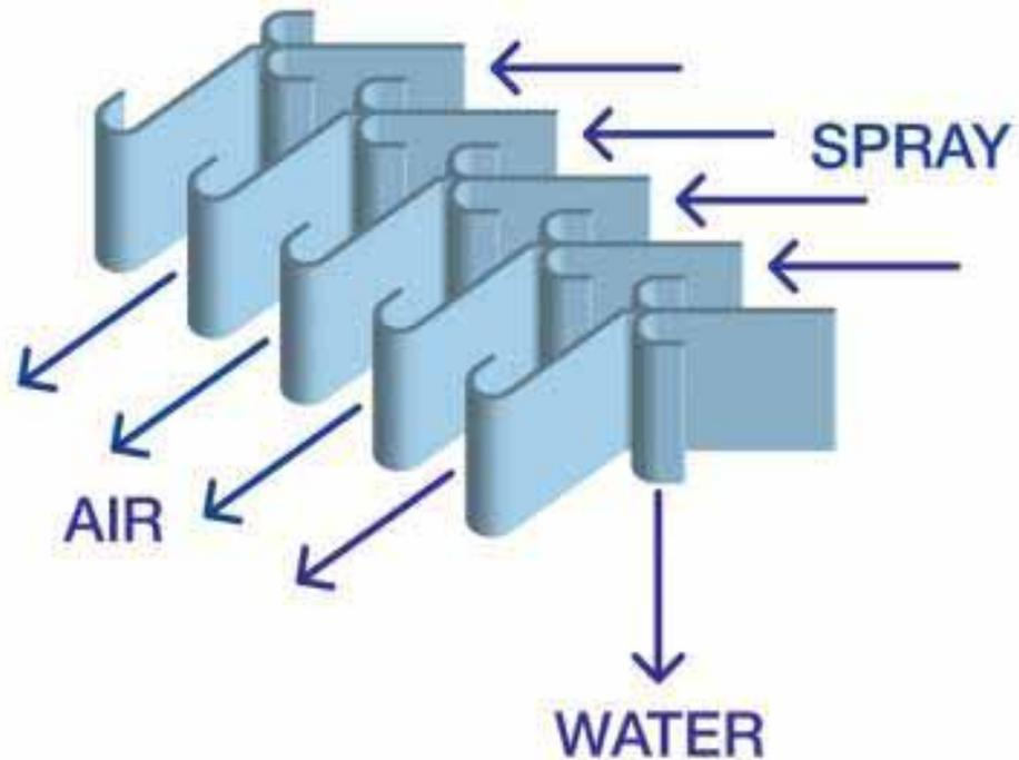
**Operation principle of Spraydown technology**
