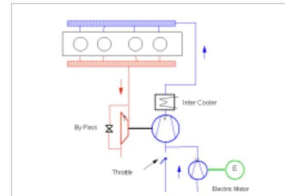
Picture: Electric assisted turbocharger
