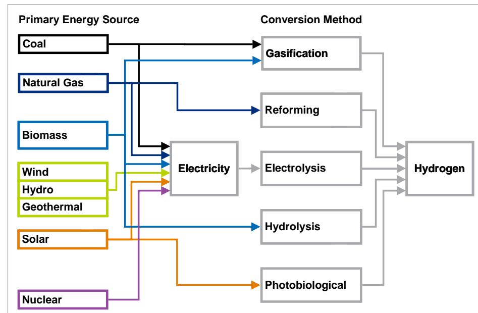
Some of the energy sources and processes that can be used to produce hydrogen
