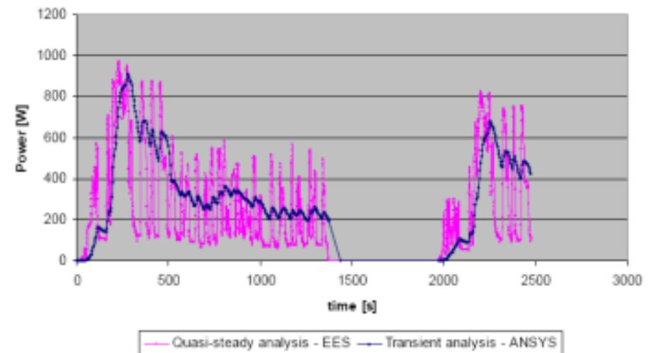
Picture: Power output SIMULATION thermoelectric generator, Ed Gundlach GM DEER 2008
