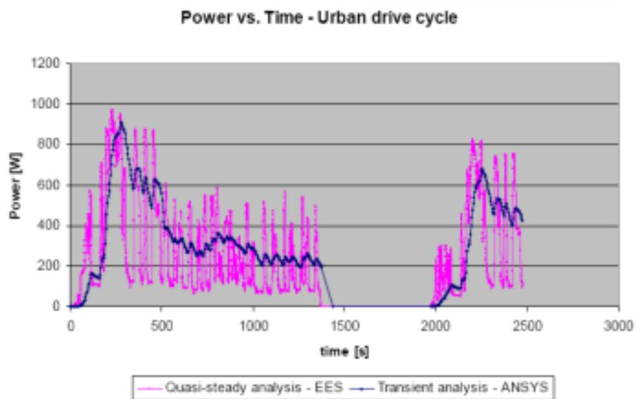
Picture: Power output SIMULATION thermoelectric generator, Ed Gundlach GM DEER 2008
