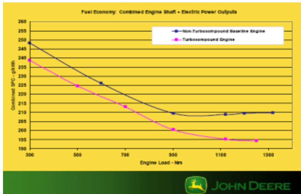
Picture: DEER 2007; Fuel consumption benefit electric turbocompound<sup>21)</sup>
