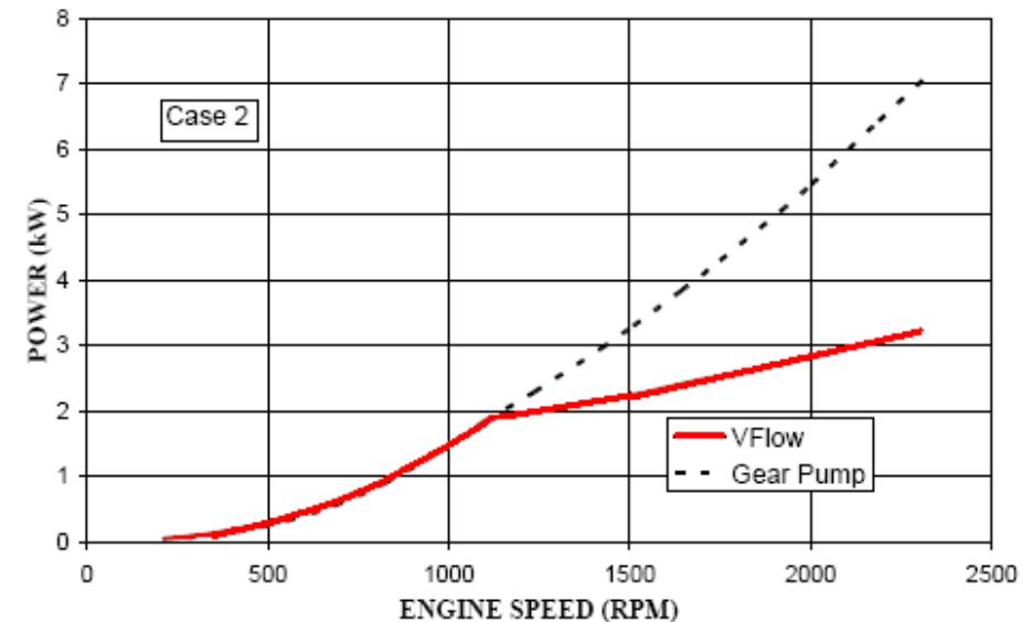
Power consumption standard gear pump and variable flow pump
