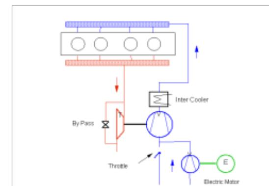
Picture: Electric assisted turbocharger
