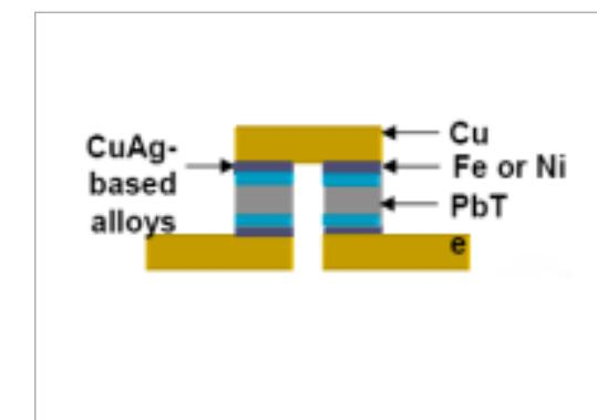
Picture: Layout thermoelectric generator,
