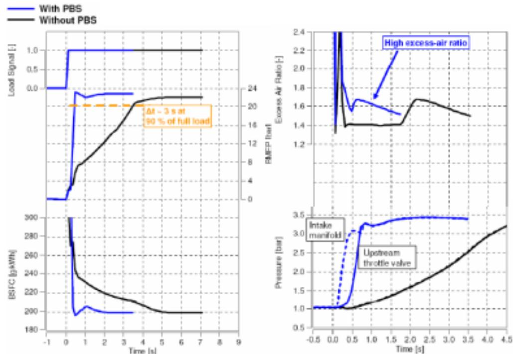
Picture: Tested PBS system at 1000rpm load response (blue PBS ON – black PBS OFF)
