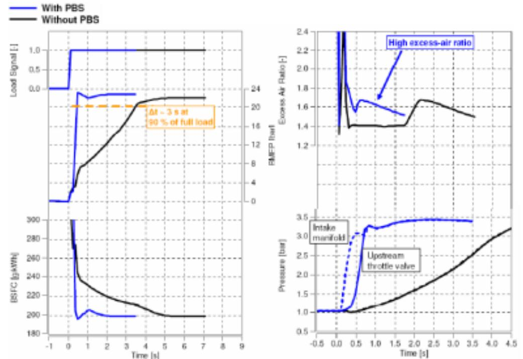
Picture: Tested PBS system at 1000rpm load response (blue PBS ON – black PBS OFF) Knorr-Bremse; 29<sup>th</sup> IWM, 2008 <sup>30)</sup>
