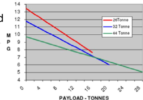
Figure: Effect on Payload on Fuel Consumption Based on 3 Different Trucks
