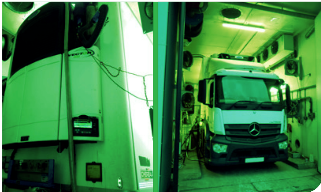
Figure 1. Semi-trailer (left) and Rigid HGV (right) and their auxTRUs
