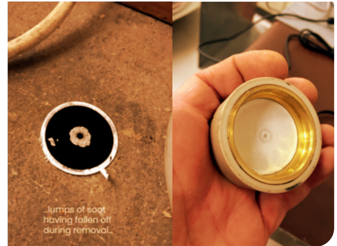
Figure 3. Filters from testing auxTRU (left) and Euro 6 diesel van (right)
