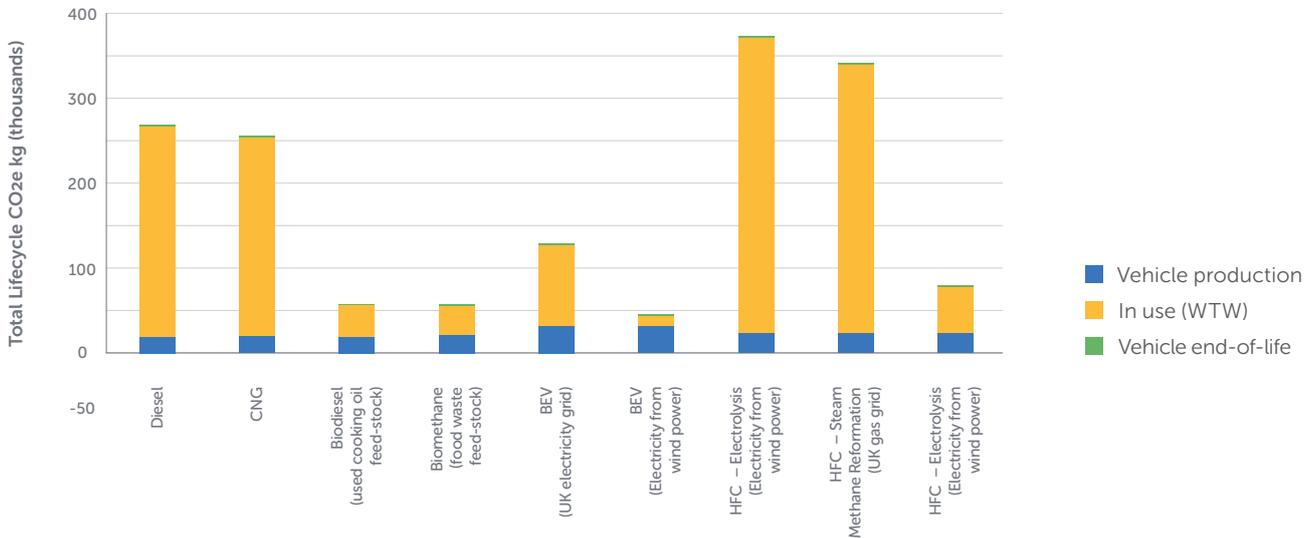
Vehicle lifecycle CO<sub>2</sub>e emissions for an urban truck across different powertrain technologies and low carbon fuels. Data supplied by LowCVP.
