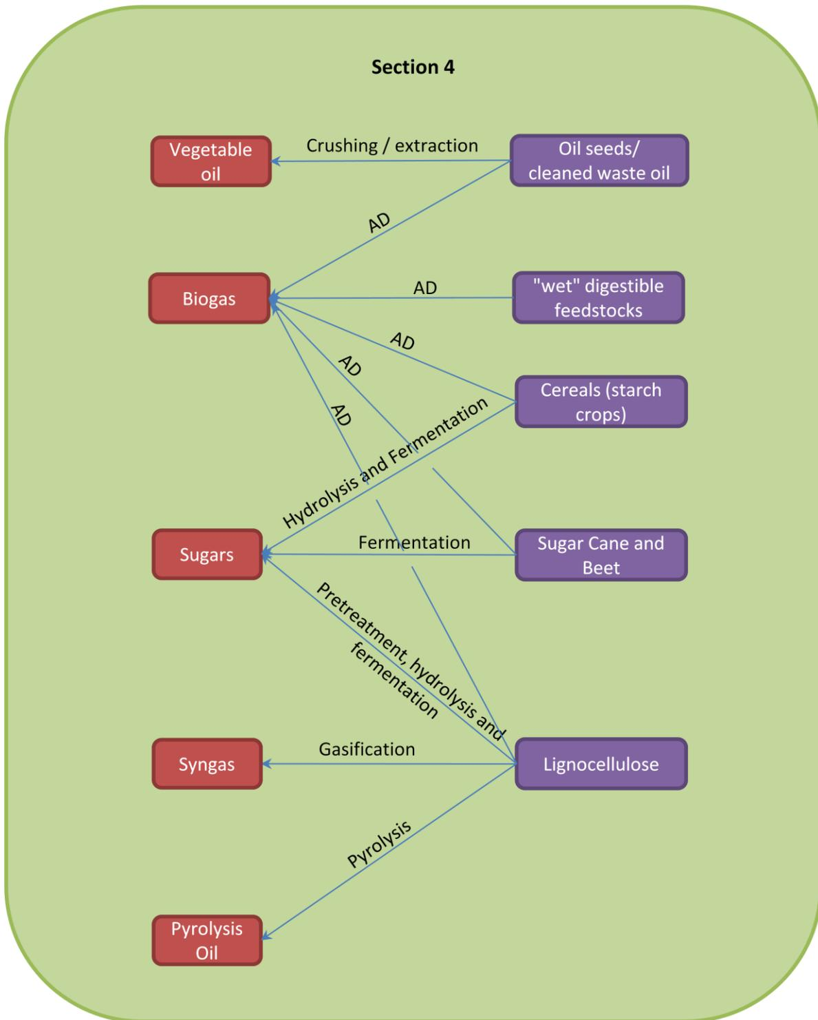
Figure 5. Feedstock conversion processes
