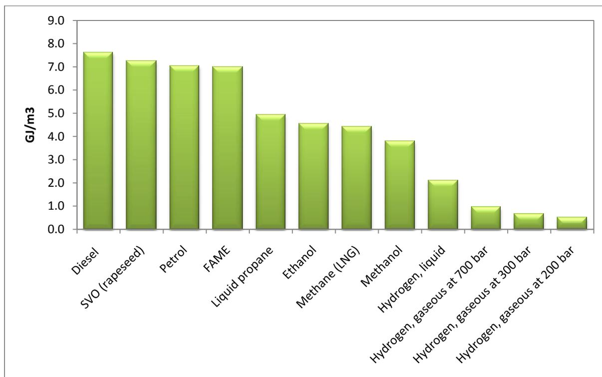
**Figure 3. Volumetric energy density of fuels adjusted for engine efficiency**
