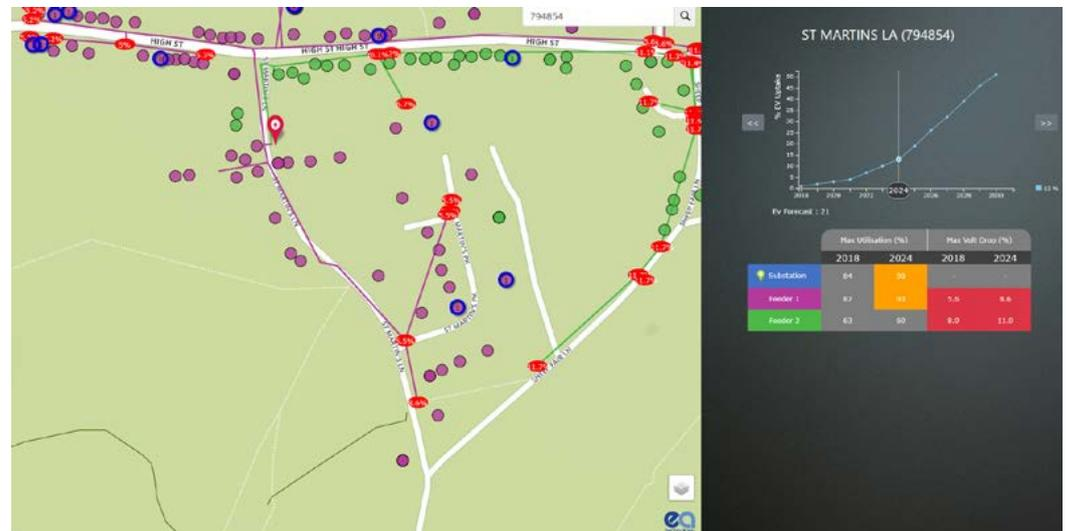
**Figure 4** Network Assessment Tool study of St Martin's Lane substation [Source: WPD]
