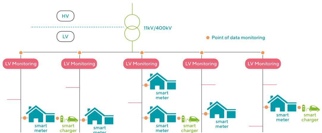
Figure 1 Different locations for monitoring the low voltage (LV) network
