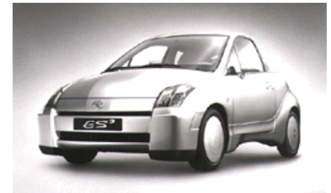
Above: Toyota's diesel hybrid test model ES3, which is capable of 47 km/l due to an efficient diesel engine and hybrid technologies
