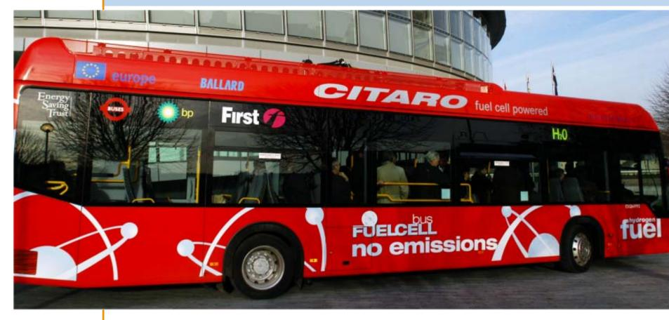
Hydrogen Fuel Cell Bus- DaimlerChrysler Citaro Prototype: Three being trialled in London 2004-5 as part of CUTE project. See www.cute-eu.net
