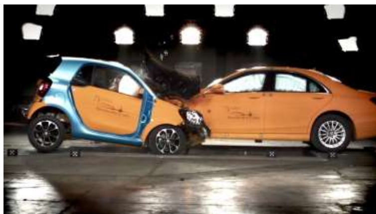
FIGURE 3.4.1 HEAD-ON SAFETY TEST BETWEEN TWO M1 PASSENGER CARS WITH MASS RATIO OF 2.5:1
