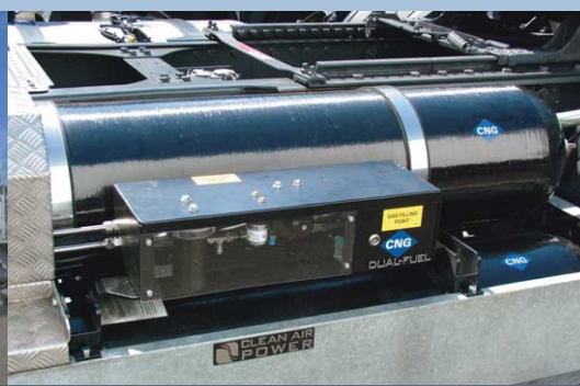
Dual fuel controls
