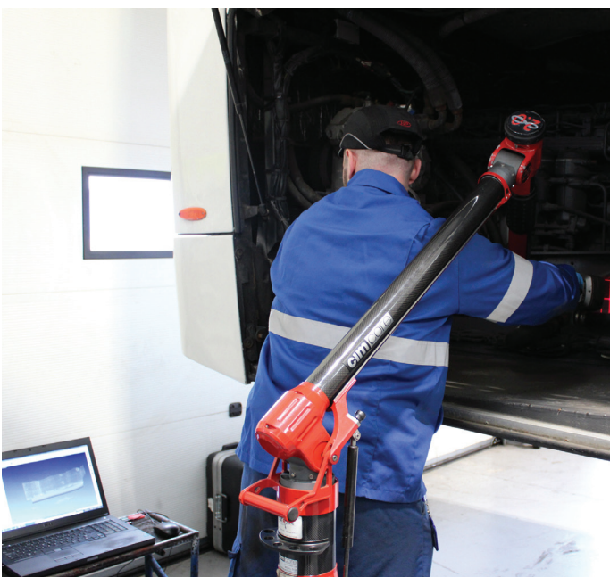
Figure 7: Technician creating 3D digital image of internal body of a coach using a laser system to identify available space for SCR system (courtesy of Eminox)
