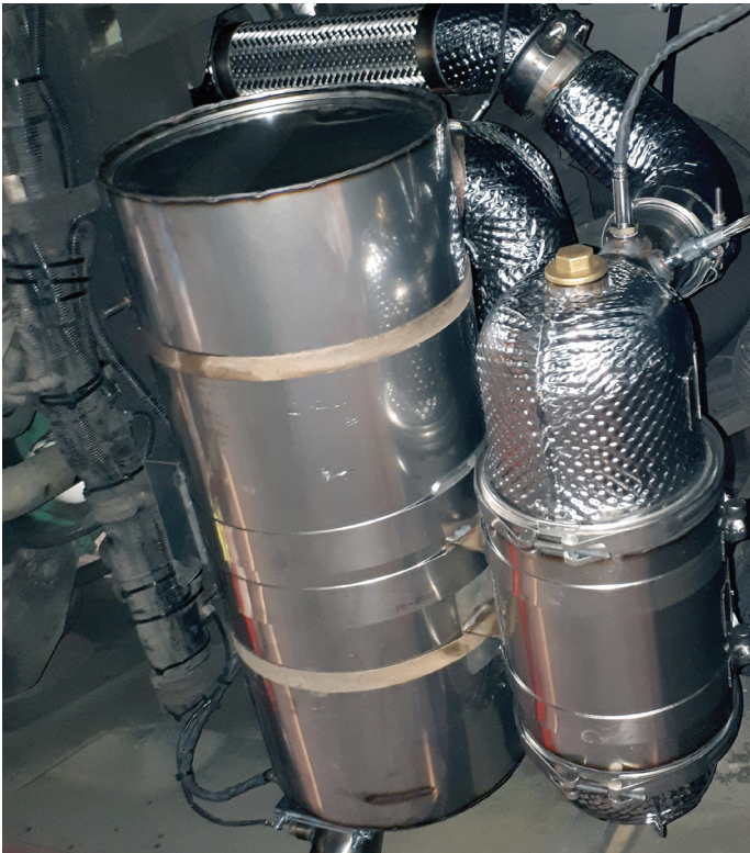
Figure 6: Proventia/Excalibre Technologies NO x BUSTER™ SCR System fitted to ADL E200 Euro V Bus
